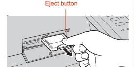
Do not remove the PCMCIA/PC Card while the Access Indicator is flashing.
